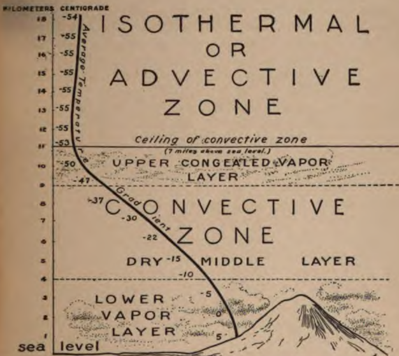
FIG. 298. — The zones of the lower atmosphere as revealed by recent kite and balloon explorations.
